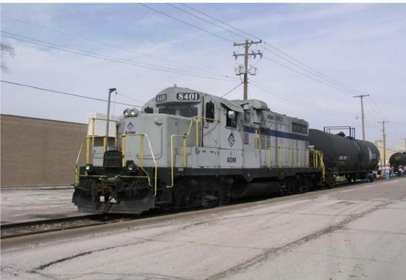
Here is a rare sight. It is ADM's Paducah Rebuild #8401 off company property. David was able to borrow the motor to pull the cars south from the wreck site. It is always easy to spot a Paducah GP 10 rebuild by the breather at the top rear of the cab and the frog-eye lights on the short hood.
