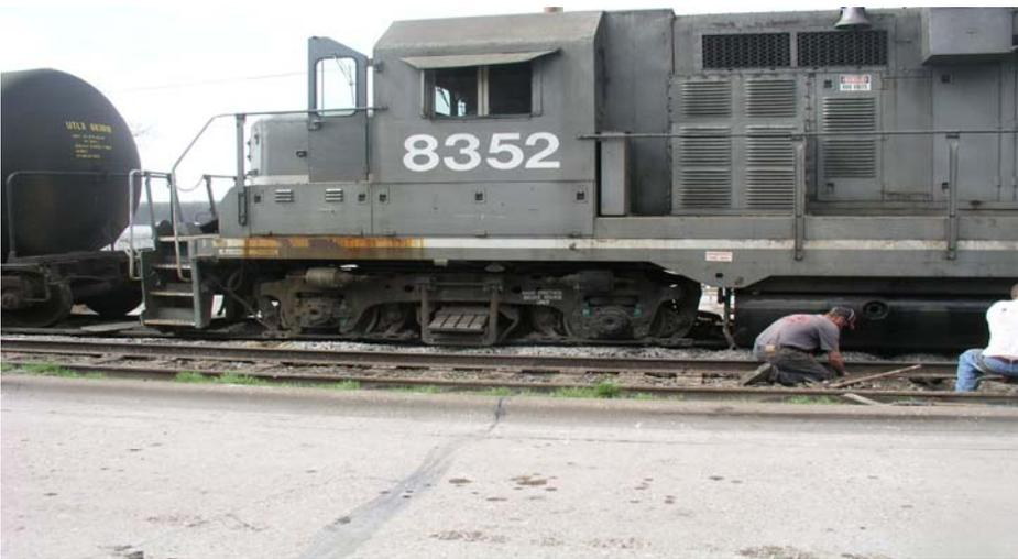
Burlington Junction's GP 11 #8352 sits with its flanges buried six inches deep in gravel along Front Street adjacent to a siding for ADM's soy oil plant.
