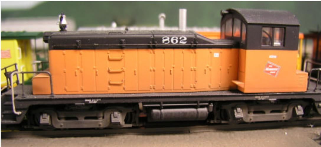
**Left;** SW1 #862. EMD built 661 of the engines between December 1938 and November of 1963. They had 567 and later 567A two stroke V-6 diesel prime movers. Each one produced 600 horsepower.
