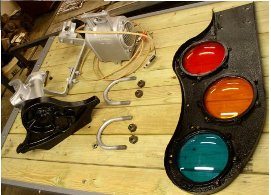
Below at left is a shot of the parts that go into creating the light housing. It's kind of like trying to put a puzzle together. Also remember that each piece had to be cleaned free of rust and assorted grime before being primed and painted.
